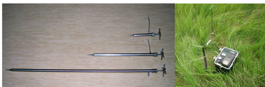
Fig. 2. The 16, 46 and 100 cm gas probes and RAD7 detector
