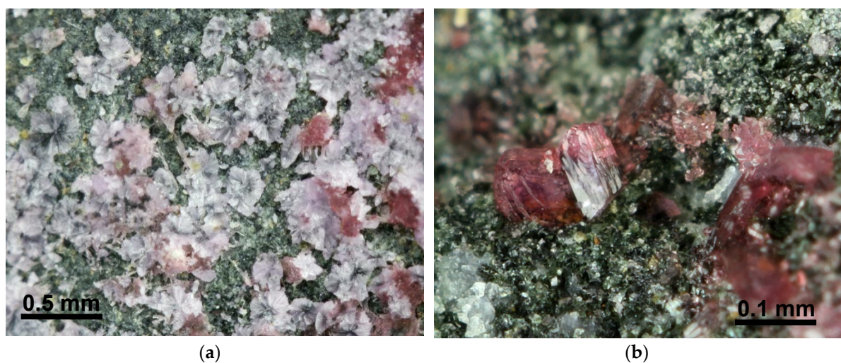
Figure 2. Variation in colour in the erythrite–köttigite series minerals from the Miedzianka polymetallic ore deposit: (a) aggregates of köttigite (colourless and white) and erythrite (pink) on the surface of chloritised amphibolite; (b) pink erythrite crystal overgrown by colourless köttigite.
