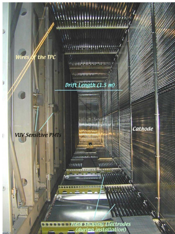
Figure 1. Cross section of ICARUS detector TPC during the assembling in Pavia, showing the field shaping electrodes, the cathode, the anodic wire planes and the PMT system.
