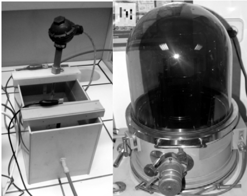
Fig. 1. Place for anodizing and Jeol IEE-4B vacuum evaporator
