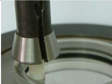
Fig. 3. Tribological pair pin on disk
