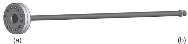
FIG. 1. The T2K replica target with the upstream aluminum flange (a) and the downstream plastic ring (b) used to support the target.
