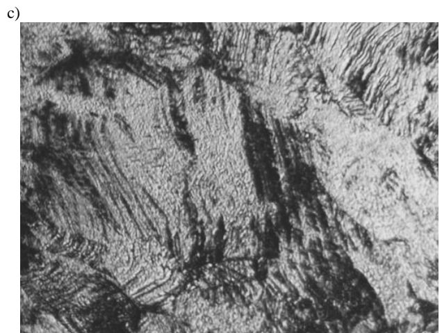
Fig. 2. Structure of the investigated steel type X5CrNi18-10 after deformation with a draft of 40%; a-c melts of these steel; Etching - Beraha's reagent, Mag. 1000x
