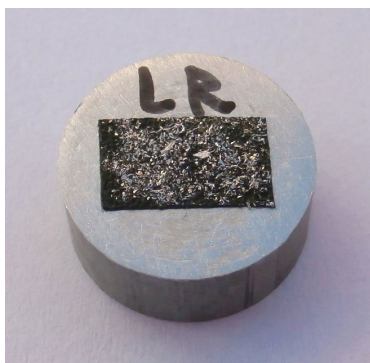
FIGURE 2. Metal waste powder collected after laser cutting (stub diameter is 12 mm).
