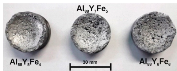
Figure 1. External morphology of \text{Al}_{88}\text{Y}_8\text{Fe}_4 , \text{Al}_{88}\text{Y}_7\text{Fe}_5 , and \text{Al}_{88}\text{Y}_6\text{Fe}_6 alloys in the form of ingots.
