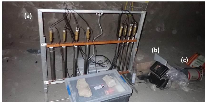
Figure 2. Measurement setup used during the measurements: (a) visible flat tray of helium counters placed vertically in the stand; visible Centronic (thicker) and ZDAJ (thinner) counters (at the base of the tray, as well as plastic boxes which are dustproof housing for DAQ (background one) and power suppliers (foreground one)); (b) radon monitor RAD7; (c) HPGe spectrometer.
