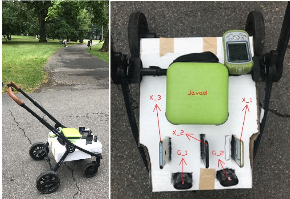
Figure 3. Survey equipment design and GNSS devices used in the study.
