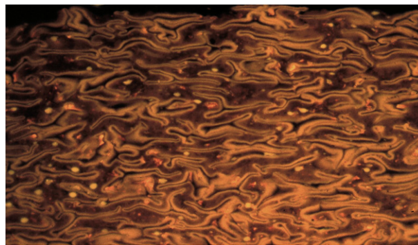
Fig. 7. (Mio-) Sporinite, Carboniferous, Saar area (Germany); fluorescence mode, width of field 180 µm. (Photomicrograph W. Pickel)
